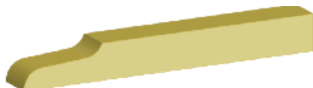
Skirting Section LADY'S SLIPPER 25 x 175mm
